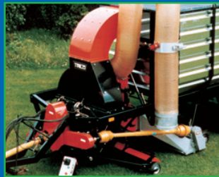
Miniflex PU-AE PU protection and suction hose, with plastic coated wire spiral, microbe resistant
